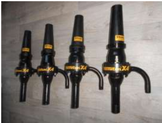
Figure 2. Shaft modification for semi-dry shotcrete
